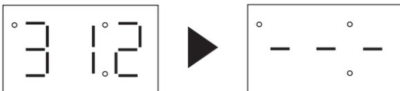
below) that identifies the parameter version contained in the drive. The display should then read "--", which indicates that the drive is in a STOP condition. This is shown below:
