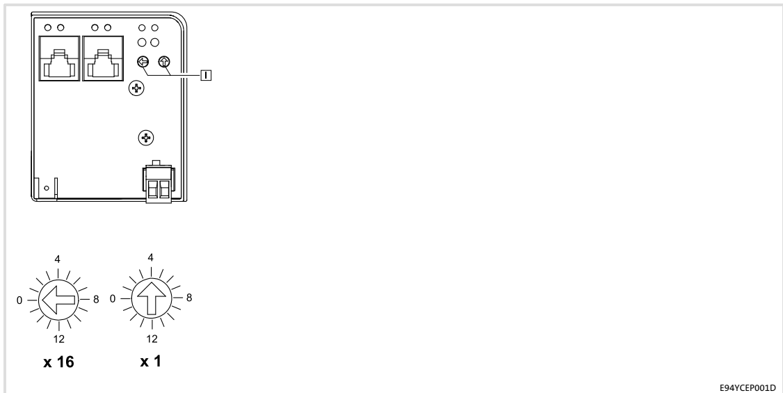
Fig. 6-1 Setting the node address
