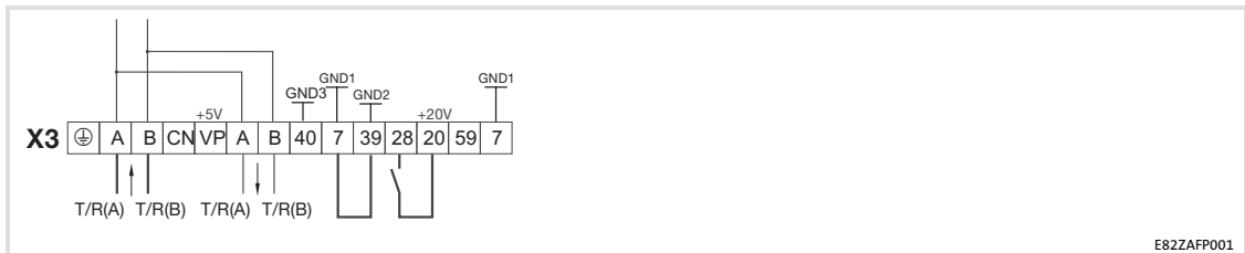
— The min. wiring requirements for operation
